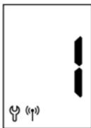
The logged-on DuoFern Room Thermostat 2 appears as “1” on the display after a successful login.
